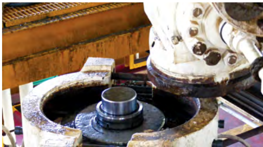
Tree removal and Tubing Hanger.
